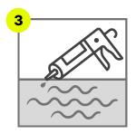
Apply Sika Dur 31 as a thinly spread layer or Hilti RE100 adhesive in this zigzags directly to surface. Make sure the full area for the mats is covered.
