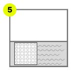
Line mat up with your desired location, ensuring the adhesive is evenly distributed along the mats under side. Press firmly onto the surface and allow to dry for four hours.
