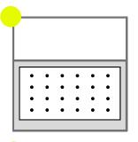
Place the drilling templates into position and tape the corners to hold in firmly in place. Ensure the template is positioned in accordance with regulations.
