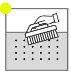
Once all the holes have been drilled to the correct depth, remove the templates. The holes and substrate must be thoroughly cleaned and dust free prior to installation of the Tactile indicators.
