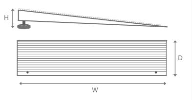
ATH1232 W=812mm, D=304mm, H=25mm - 50mm ATH1236 W=914mm, D=304mm, H=25mm - 50mm ATH2432 W=812mm, D=610mm, H=50mm - 89mm ATH2436 W=914mm, D=610mm, H=50mm - 89mm ATH3632 W=812mm, D=914mm, H=89mm - 127mm ATH3636 W=914mm, D=914mm, H=89mm - 127mm ATH4832 W=812mm, D=1219mm, H=101mm - 152mm
